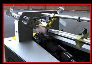
A movable end-stop and proximity sensor allows the user to fully customise tube length and louver patch length
