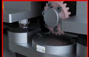
Precision linear bearings with reticulating ball bearings running on hardened ground guide-ways ensure smooth operation, and a cutter angle plate ensures accurate setup.
