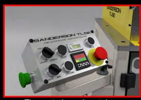
The control panel contains a programmable louver counter, an easily resettable parts counter, and a toggle between louver punch count and louver patch length
